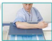
Wireless mode enables free positioning with easy handling. When used as a wireless portable type, table-top exposures are easily performed, allowing exposure situations to be expanded.
