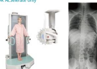
The Automatic Image Stitching combines multiple images into a single image for viewing a wide area.
